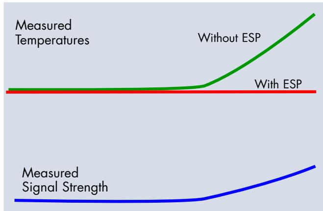
**Ladle Reflections:** As a ladle is tipped, hot refractory walls are exposed, and a reflected image of these walls can cause a sensor without ESP to read in error. By monitoring the increase in signal strength, the sensor with ESP can recognize the presence of reflections and maintain an accurate measurement.
