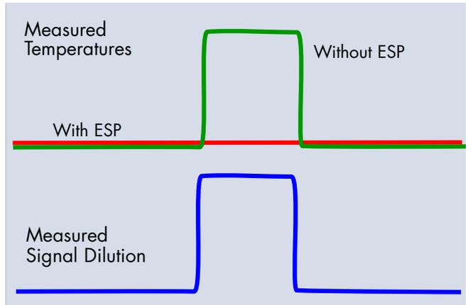
**Sparklers:** As molten iron cools, carbon comes out of suspension and ignites to create sparklers that cause a sensor without ESP to read too high. By monitoring the increase in signal dilution, the sensor with ESP can recognize the presence of the sparklers and maintain an accurate measurement.
