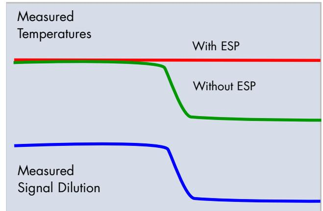
**Heavy Smoke:** Heavy smoke can obstruct the sensor's view of the measured target and cause a sensor without ESP to read in error. By monitoring the decrease in signal dilution, the sensor with ESP can recognize the presence of smoke and maintain an accurate measurement.
