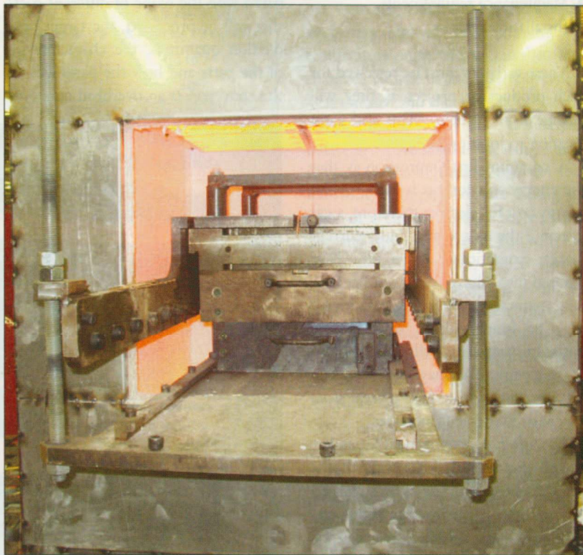
Infrared is used to preheat a heavy metal mold, maintaining close temperature tolerance through the mold mass.
